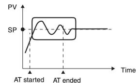
method (called the limit cycle method) for forcibly changing the manipulated variable and finding the characteristics of the control object is employed.
