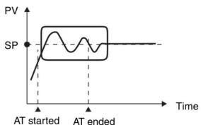
Set the HY is  $0.5\sim1^{\circ}$ C, if the output is relay set the t=10S, then set the AT=1, the lamp of AT will be flashed, in this time the controller enter into **Auto-tuning**. now meter's control way is on-off mode, after 3 times vibrating( 3 control period) automatically save P, I, D parameter, the self-adjusting procession finished.
