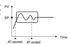
changing the manipulated variable and finding the characteristics of the control object is employed.
